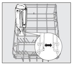
Place the bottle holder in the position shown in the bottom basket. If placed anywhere else, water will not be able to access the bottle properly, and cleaning results will be impaired.
